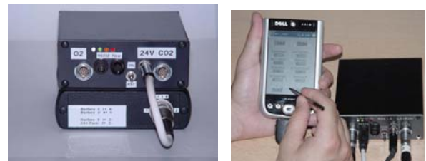
Fig. 27: Electronic unit in current status (PRO1.5) with rechargeable battery pack for an operation time of about 3 hours (left) and communication between the PDA and the RSS-EB (right)
