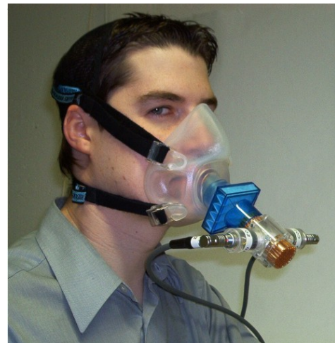
Fig. 35: The respiratory sensor system – current status. A potential safety risk exists in case of sensor breaking (A: inspiration, B: expiration). Note: Sensor design (especially heater) is optimised to induce minimum thermal stress. After approx. 5 years of sensor testing, having investigated >2.000 sensors, not a single break-up occurred.
